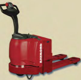
Model 8300 Walkie Pallet Truck 6,000 lb. capacity
