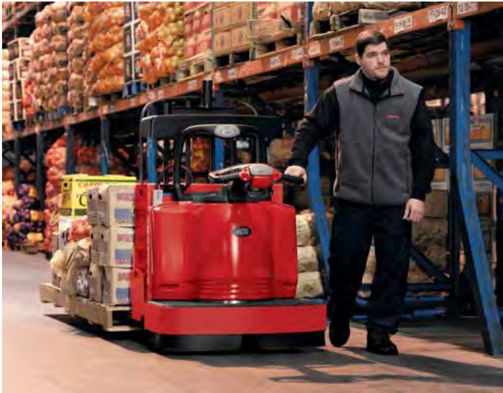
Raymond's CoastPro™ system can be activated with only one hand, for faster order picking.
