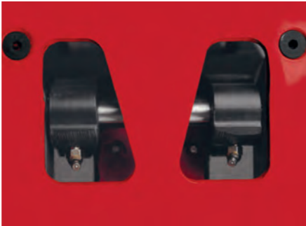
New access holes allow easier load wheel maintenance, and conveniently placed grease fittings simplify lubrication.
